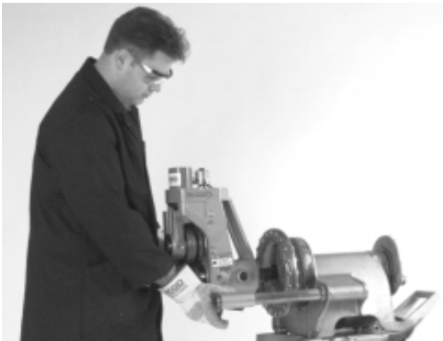
Figure 2 – Installing on 300 Power Drive
