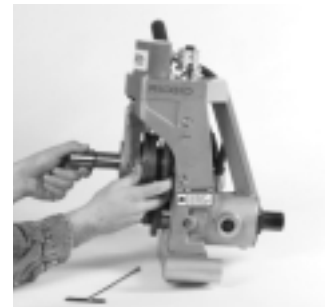
Figure 18 – Removing Retaining Shaft and Groove Roll
