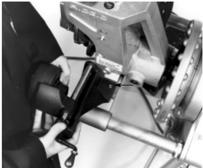
Figure 22 – Line Up Bolt Holes in the Mounting Bracket with Bolt Holes in the Base
