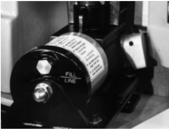
Figure 24 – Reservoir Filler Cap
