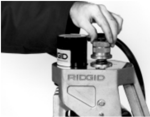
Figure 14 – Close-Up of Depth Adjustment Knob Backed Up with Gap Between Bottom of Knob and Casting
