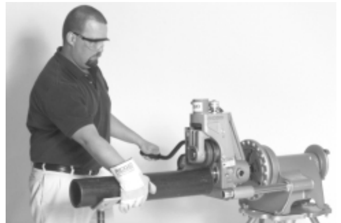
Figure 16 – Applying Pressure on Pipe with Power Drive in REV Mode.
