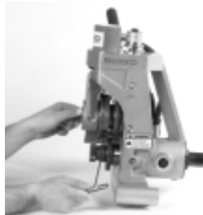
Figure 17 – Loosening Grooving Roll Set Screw
