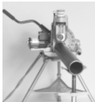
Figure 12 – Offset Pipe on 918 in FORWARD Position
