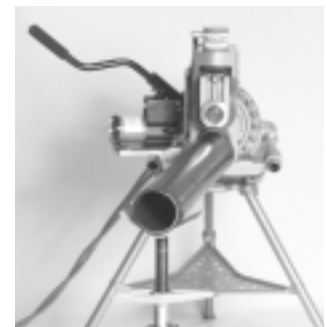
Figure 13 – Offset Pipe on 918 in REVERSE Position
