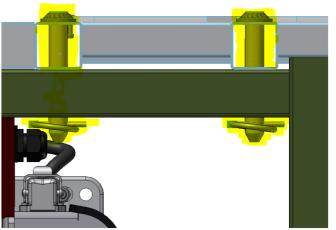
Depending on the width of the platform (W), a part of the roof can be folded upwards.
