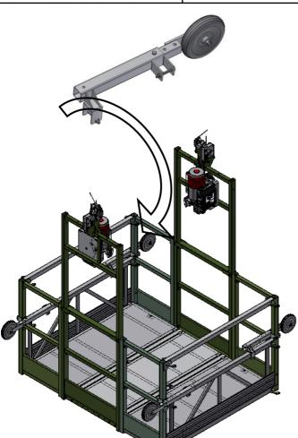
Install and tighten (2 times 4 HM10x30 bolts and locknuts) the bottom guides beam with wheels:
