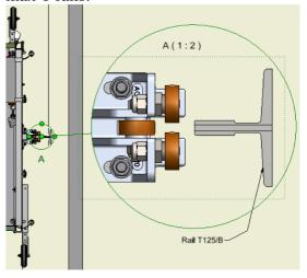
Install and tighten the two bottom guides on the baseboards of the site supports
