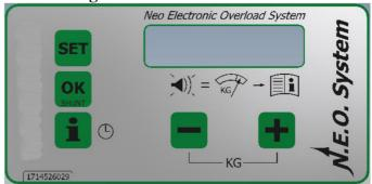
A load control feature is included in the e.lift 600 hoist. It allows you to stop the lifting and lowering movement of the hoist before the load reaches 125% of the selected setting.
